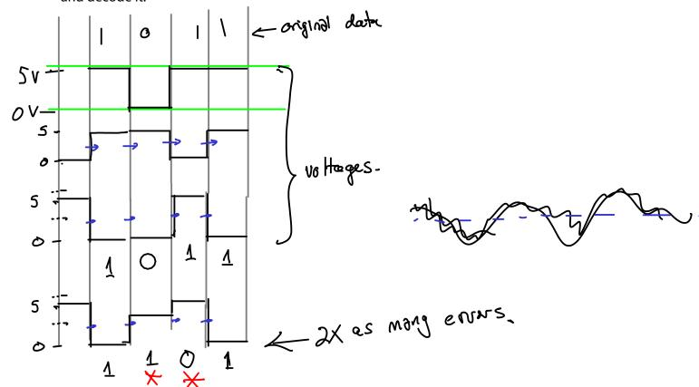
Exercise 4: How many combinations are there of 3 bits? Of 4 bits? How many bits might be input and output by an 8B10B code? What might a 4B3T code mean?
