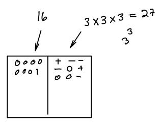
**Exercise 5**: Design your own 2B3B line code by choosing the output waveforms that have the lowest average DC value and giving preference to those that start and end at different levels (assume bipolar signalling).
