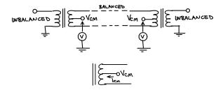
**Exercise 6:** If the common-mode circuit is used to carry 500mA, how much current flows through each half of the transformer secondary? What is the net effect on the flux in the transformer core?
