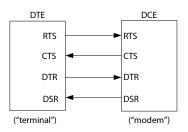
The second set of control signals are DTR (Data Terminal Ready) and DSR (Data Set Ready). These signals indicate that the DTE and DCE devices respectively are connected and operational. Typically they indicate that the power is turned on. However, by de-asserting DTR it is possible, if the modem is correctly configured, for the DTE to prevent the DCE from sending data on RxD.
