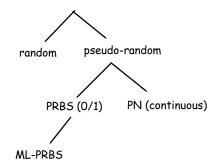
PN and PRBS signals have many important applications in communications systems. In this lecture we will study the properties of a type of PRBS called a maximal-length (ML) sequence, learn how to generate these sequences and look at one of their applications – "scrambling." Other applications include spread-spectrum systems and the generation of test signals. ML PRBS sequences, sometimes called m-sequences, have a number of interesting properties including:
