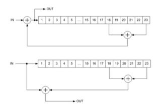
One problem with self-synchronizing scramblers is that an error in the received data pattern can result in multiple errors in the de-scrambled data. This is called error propagation.
