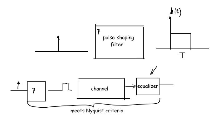
**Exercise 5**: Draw the impulse response of a filter than converts input impulses to pulses of duration T? What is the shape
