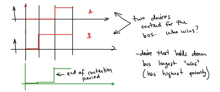
**Exercise 5**: Consider a communication bus in a car that connects an airbag activation controller with a collision detector, a passenger-seat occupancy sensor and an airbag-disabling switch. Would it be more appropriate to use a polling- or contention-based bus arbitration protocol? Would it be appropriate for the arbitration protocol to allow different priorities for bus access? If so, what priorities might be assigned the different sensors?
