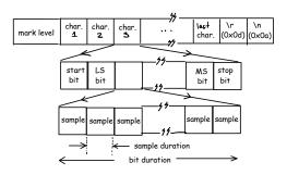
A diagram summarizing the format of the RS-232 waveform for one character is shown below.
