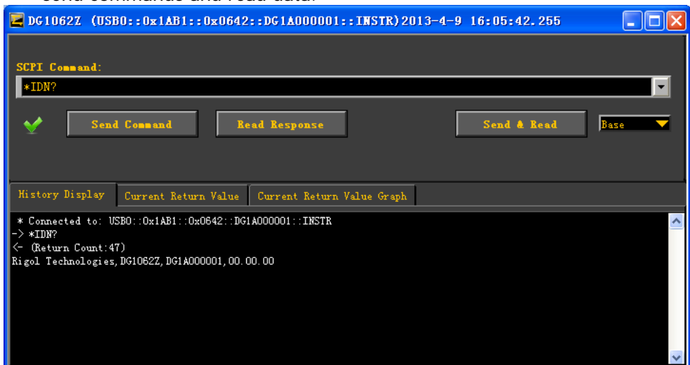
Figure 12 Send and Read Commands via USB
