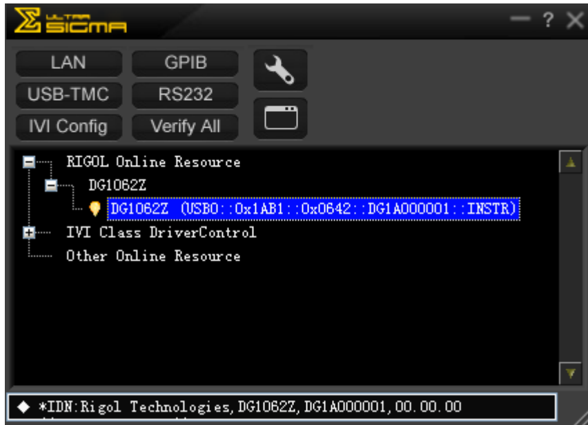
Figure 11 To View USB Instrument Resource
