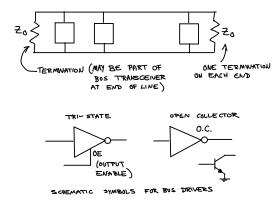
RS-485 is a standard similar to RS-422 that allows multiple drivers to be connected to a multi-drop bus. Only one device can have an active output at any given time – the others must be in a high-impedance mode.
