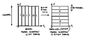
The reduction in symbol rate (or increase in symbol period) reduces the impact of ISI because the impulse response of the channel is now a shorter fraction of the symbol period. Most OFDM systems also
