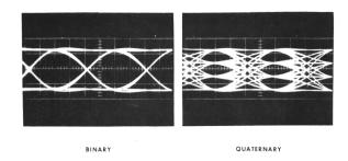
The vertical opening at the sampling time, called the "eye opening", represents the amount of ISI at the sampling point.
