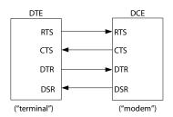
The second set of control signals are DTR (Data Terminal Ready) and DSR (Data Set Ready). These signals indicate that the DTE and DCE devices respectively are connected and operational. Typically they indicate that the power is turned on.
