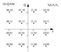
where each point is labelled with the bits that are transmitted if that symbol (a carrier with the given I and Q amplitudes) is transmitted.
