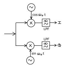
The receiver has to recover the phase of the carrier to accurately set the I and Q phases. This can be done, for example, by transmitting a preamble that is used as the phase reference for the rest of the frame.
