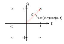
**Exercise 2**: Label the other three points in the constellation diagram with the equation of the signal that corresponds to that point.
