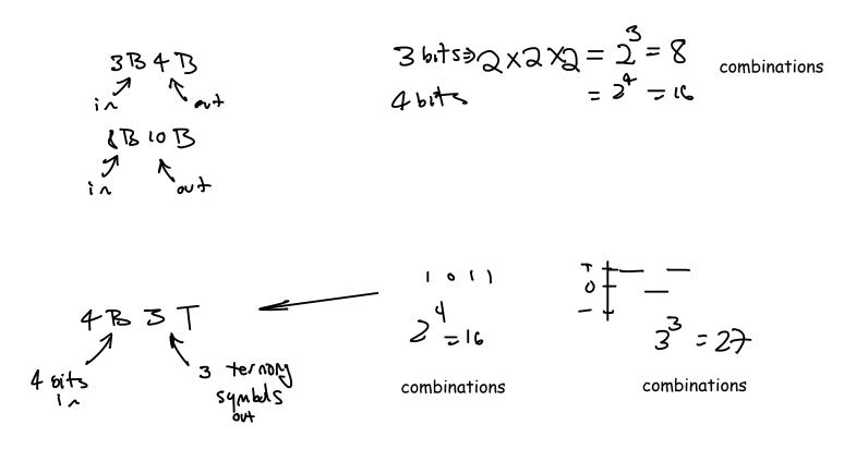
**Exercise 5**: Design your own 2B3B line code by choosing the output waveforms that have the lowest average DC value and giving preference to those that start and end at different levels (assume bipolar signalling).
