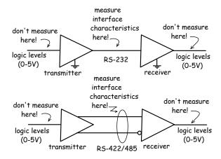
The ICL-232 includes two line drivers (transmitters) and two receivers. You can test any pair. The MC3487 and MC3486 include four drivers or receivers. You can measure any one of the four.
