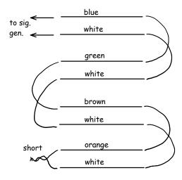
• increase the frequency until the signal level is minimum. If you have one of the longer lengths of cable you might see multiple nulls; use the first (lowest frequency) null to compute the length.
