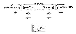
**Exercise 2:** If the common-mode circuit is used to carry 500mA, how much current flows through each half of the transformer secondary? What is the net effect on the flux in the transformer core?
