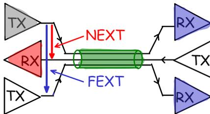
Note that the coupling between pairs in a cable happens throughout the length of the cable. The difference between NEXT and FEXT is in which receiver is affected (the near one or the far one), not where the coupling takes place.
