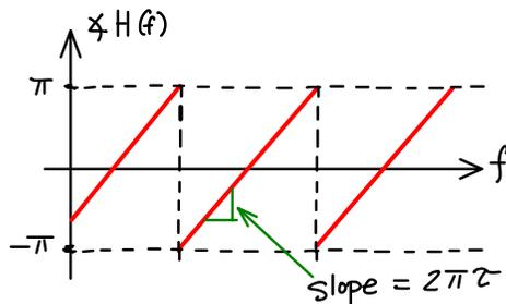
**Exercise 1:** A 100m transmission line has a velocity factor of 0.66. Plot the phase response of the cable over the frequency range 0 to 6 MHz.
