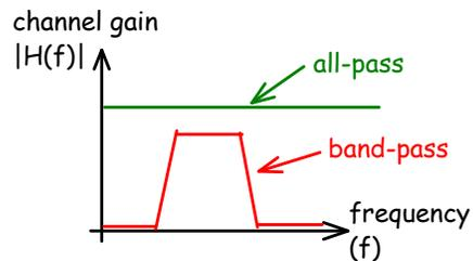
Channels often include several of the above characteristics. For example, a twisted pair loop may include a notch filter to remove 50Hz or 60Hz power line noise, it may have peaks and valleys in the frequency response due to reflections from taps or poor terminations and it will drop off with frequency due to higher losses at higher frequencies.
