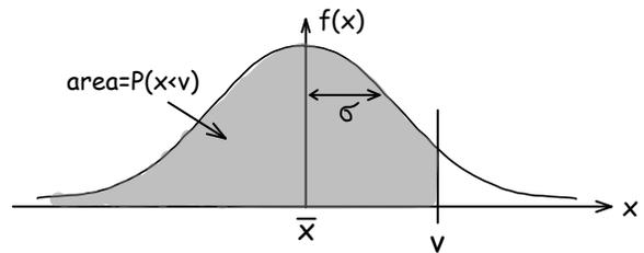
It's often useful to know the probability that the voltage of a Gaussian noise signal will exceed a certain voltage. If the signal  $x$  has a DC (mean) value  $\bar{x}$  and an RMS AC voltage  $\sigma$  then the probability that the noise voltage is less than  $v$  is given by the Gaussian (Normal) cumulative distribution function (CDF). This is the area under the Gaussian distribution curve to the left of (less than) the value  $v$ .
