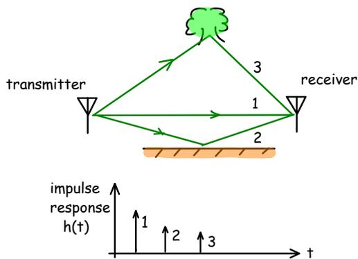
Since the each path length can be different, the delays for each path can be different. The different paths can add up constructively or destructively depending on the frequency and the delay. The frequency response can thus have peaks and nulls.
