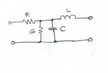
and the complete transmission line as an infinite sequence of the above blocks:
