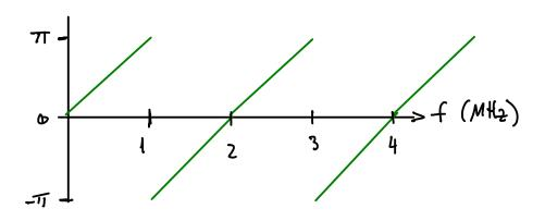
**Exercise 2**: A telephone line is being used to transmit symbols at a rate of 300 symbols/second. If the group delay must be less than 10% of the symbol period, what is the maximum allowable group delay?
