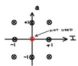
The amplitude of a vector (or the sinusoid represented by a vector) is its length. The center point represents a vector or zero amplitude and would not be used as specified in the question and as shown above. This leaves 8 constellation points which represent the 8 possible transmitted symbols. With 8 symbols we can transmit  $\log_2 8 = 3$  bits per symbol.
