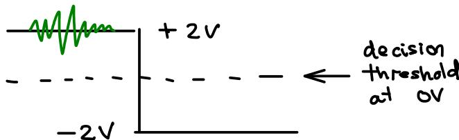
noise margin is voltage required to cause an error = 2V
