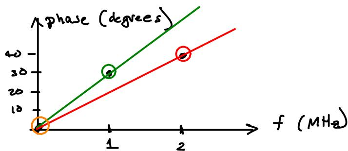
thus the channel is not linear phase and will distort signals passed through it that have frequency components in this range (for example, a  $\mu\text{s}$  pulse).
