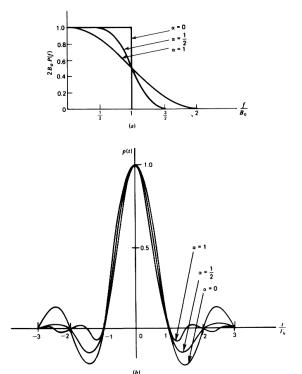
Larger values of excess bandwidth result in smaller values of the impulse response which in turn reduces the amount of ISI near the sampling point. This makes the receiver less sensitive to errors in the timing of the sampling point.
