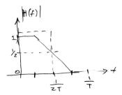
The dashed line is a "brick-wall" filter whose response is 1 below half of the symbol rate and zero above that. Although such a filter would have the minimum overall bandwidth, it is not physically realizable and has other problems as described below.
