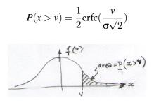
**Exercise 6**: The output of a noise source has a Gaussian (normally) distributed output voltage. The (rms) output power is 20mW and the output impedance is 100 $\Omega$ . What fraction of the time does the output voltage exceed 300mV? Hint: the variance ( $\sigma^2$ ) of a signal is the same as the square of its RMS voltage.
