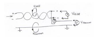
The loops between the wires are much smaller. In addition, the voltages induced on the twisted pair will mostly cancel out due to the twisting. A properly-designed receiver can ignore the common-mode voltage.
