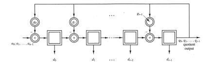
holds the result of the intermediate remainder after each subtraction. The shift register only has to hold (n-k) bits.
