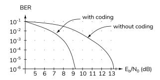
What is the coding gain at a BER of  $1 \times 10^{-3}$ ?
