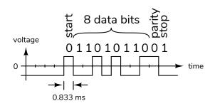
For the first version, the data bits, in order from m.s.b. to l.s.b. are 0110 1001 which is 0x69.
