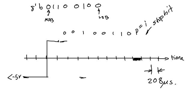
**Exercise 5**: What happens if the receiver's clock is running faster than the transmitter clock?
