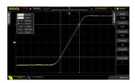
Take a screen capture of the 'scope output showing the waveform and the measurements. Calculate the slew rate. Does it meet the ICL-232 specification(s)?
