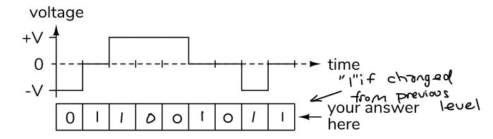
(b) The diagram below shows a data signal encoded using a *differential* Manchester line code following the conventions in the lecture notes. Fill in the boxes with the bit values that were being transmitted in each time interval.
