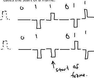
**Exercise 2**: Preambles such as this allow multiple transmission formats to be used in a backwards-compatible way. What might be some disadvantages of using such a preamble? *Hint: to be decoded by old ("legacy") devices the preamble must be transmitted at the lowest possible data rate. This can be 100 times slower than the fastest devices.*
