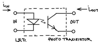
Since the connection between the LED and photodiode is by light alone, the input and output can be completely isolated electrically. The two sides do not even have to share a ground connection.
