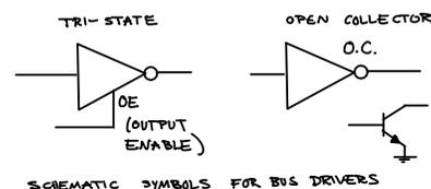
RS-485 is a standard similar to RS-422 that allows multiple drivers to be connected to a multi-drop bus. Only one device can have an active output at any given time – the others must be in a high-impedance mode.
