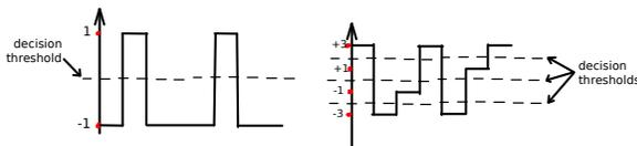
A circuit called a comparator could be used to convert the analog input to a digital (logic-level) signal. If the symbols are at more than two levels we would need more than one comparator and some logic (e.g. a priority encoder) to convert the input level to a multi-bit digital output.
