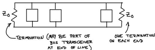
Passive terminations are resistors of a resistance equal to the characteristic impedance of the transmission line.
