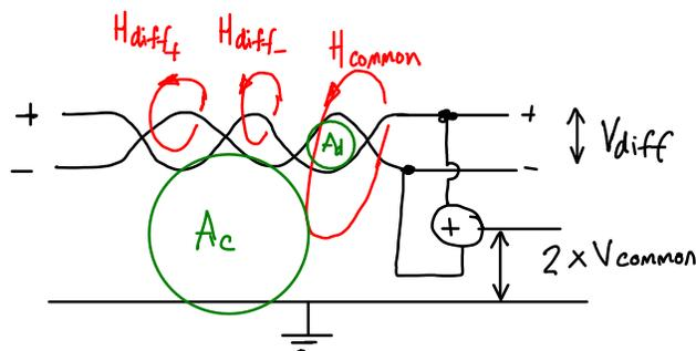
The two conductors of the twisted pair are next to each other and the area between the wires ( $A_d$ ) is much smaller than the area between the wires and ground ( $A_c$ ). This will result in a smaller voltage being induced on the differential signal. In addition, the voltages induced on the twisted pair by the magnetic field (the parts of the field  $H_{diff+}$  and  $H_{diff-}$ ) will cancel out due to the twisting.
