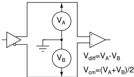
A differential transmitter encodes data as the differential voltage – the voltage difference between its two outputs. For example,  $V_A = +5\text{ V}$  and  $V_B = 0\text{ V}$  for a logical '1' and  $V_A = 0\text{ V}$  and  $V_B = +5\text{ V}$  for a logical '0'.
