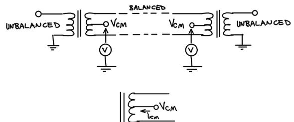
**Exercise 8:** If the common-mode circuit is used to carry 500mA, how much current flows through each half of the transformer secondary? What is the net effect on the flux in the transformer core?
