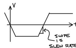
**Exercise 4:** The RS-232 standard specifies a maximum slew rate of  $30V/\mu s$ . Assuming a voltage swing of 30 volts, what is the maximum
