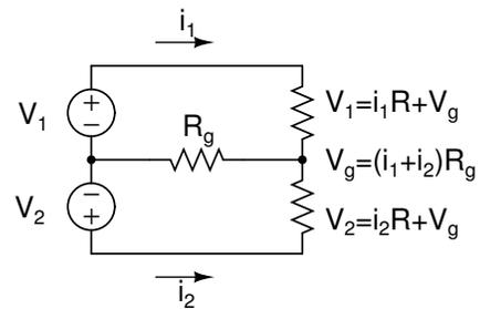
These effects can be particularly severe when the shared ground circuit is used as the return path for a power supply.
