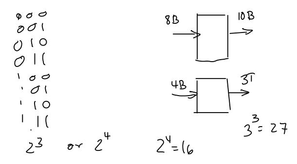
**Exercise 7**: Design your own 2B3B line code by choosing the output waveforms that have the lowest average DC value and giving preference to those that start and end at different levels (assume bipolar signalling).
