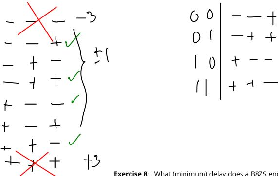
**Exercise 8**: What (minimum) delay does a B8ZS encoder add? Receiver? Why is there a zero between successive same-polarity pulses?
