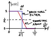
The "brick-wall" filter (blue) has a response that is 1 below half of the symbol rate  $(\frac{1}{2} \cdot \frac{1}{T} = \frac{1}{2T}$  where  $\frac{1}{T}$  is the symbol rate) and zero above that. Although such a filter would have the minimum bandwidth required to meet the Nyquist condition for a symbol period *T*, it cannot be built because the delay through the channel would be infinite.
