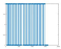
Check the waveform at this point to make sure at least the start and end polarity are correct and you have approximately the right number of samples (number of characters × number of bits per character × number of samples per bit). Use File > Save to save it to a format that you can include in your report (e.g. .png).
