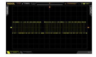
Set up serial protocol decoding as in the previous lab but use the ascii format display for this lab so you can see the characters in the string being transmitted.
