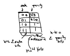
**Exercise 6**: The data rate over the channel is 50 Mb/s; a rate 1/2 code is used. What is the throughput?
