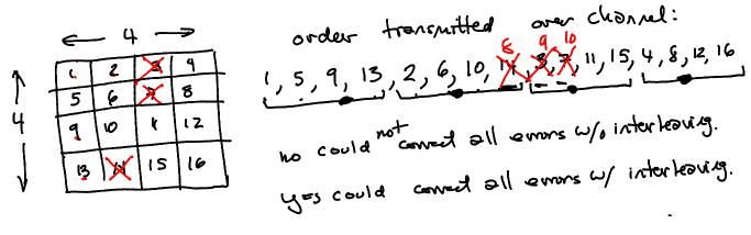
**Exercise 15**: If errors on the channel happened in bursts and you were using a RS code using 8-bit words, would you want to interleave bits or bytes?
