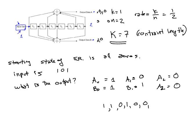
**Exercise 12**: Consider the encoder above. If the only the bits corresponding to the outputs A, A and B, and B are transmitted corresponding to every three input bits, what is the code rate of this punctured code?
