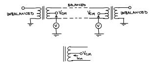
**Exercise 8:** If the common-mode circuit is used to carry 500mA, how much current flows through each half of the transformer secondary? What is the net effect on the flux in the transformer core?
