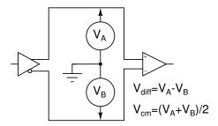
A differential transmitter encodes data as the differential voltage – the voltage difference between its two outputs. For example,  $V_A = +5$  V and  $V_B = 0$  V for a logical '1' and  $V_A = 0$  V and  $V_B = +5$  V for a logical '0'.
