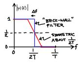
The "brick-wall" filter (blue) has a response that is 1 below half of the symbol rate  $(\frac{1}{2} \cdot \frac{1}{T} = \frac{1}{2T})$  where  $\frac{1}{T}$  is the symbol rate) and zero above that. Although such a filter would have the minimum bandwidth required to meet the Nyquist condition for a symbol period T, it is not physically realizable. The filter with the straight-line transfer function would be more practical.
