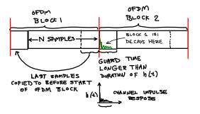
The value of N is typically a power of 2 to allow efficient implementation using the Fast Fourier Transform (FFT) algorithm.
