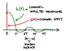
**Exercise 2:** What is the impulse response of a channel that does not alter its input? Does this impulse response meet the Nyquist condition? Will it result in ISI?
