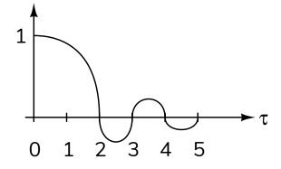
A channel has the impulse response shown above. The time axis units are microseconds. What is the maximum symbol rate that can be transmitted over this channel without ISI?
