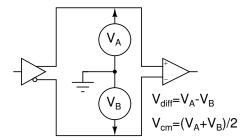
A differential transmitter encodes data as the differential voltage – the voltage difference between its two outputs. For example,  $V_A = +5$  V and  $V_B = 0$  V for a logical '1' and  $V_A = 0$  V and  $V_B = +5$  V for a logical '0'.
