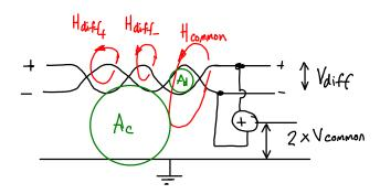
The two conductors of the twisted pair are next to each other and the area between the wires  $(A_d)$  is much smaller than the area between the wires and ground  $(A_c)$ . This will result in a smaller voltage being induced on the differential signal. In addition, the voltages induced on the twisted pair by the magnetic field (the parts of the field  $H_{\rm diff+}$  and  $H_{\rm diff-}$ ) will cancel out due to the twisting.
