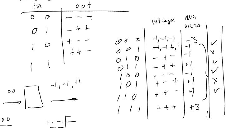
**Exercise 8**: What (minimum) delay does a B8ZS encoder add? Receiver? Why is there a zero between successive same-polarity pulses?
