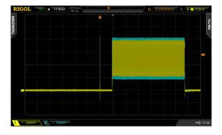
Enable the Math channel and display the differential voltage (A-B with A as channel 1 and B as channel 2) as well as the two AWG channels superimposed. The initial portion of the frame should something like:
