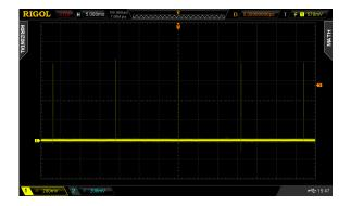
and each frame should be preceded by a normal link pulse:
