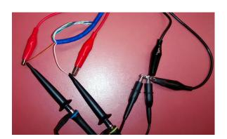
Use the oscilloscope to check that the voltage levels, signal period and the preamble waveform are as expected.
