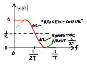
Note that it is the symmetry around the frequency  $\frac{1}{2T}$  that ensures there will be no ISI rather than the exact filter shape. Thus we are free to implement other transfer functions if they make the implementation easier.
