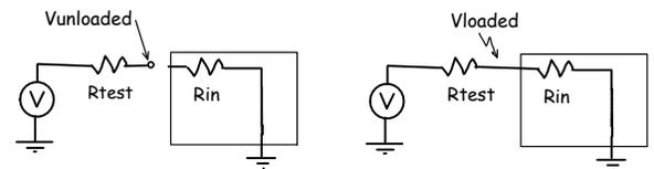
However, note that the output voltage versus current characteristic may not be linear and so the apparent input and output impedances may depend on the current. You should make the measurements at the test conditions specified in the datasheet.
