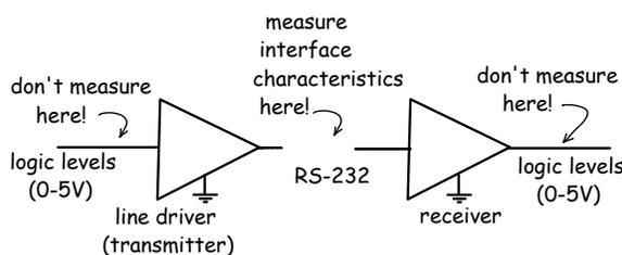
The ICL-232 includes two line drivers (transmitters) and two receivers. You can test either of the transmitters and either of the receivers.
