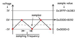
The samples values in the .raf file must be in "little-endian" byte order – the least-significant byte of each two-byte word should appear first. The contents of the file for the waveform above would be as shown in the following hex dump:
