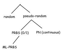
PN and PRBS signals have many important applications in communications systems. In this lecture we will study the properties of a type of PRBS called a maximal-length (ML) sequence, learn how to generate these sequences and look at one of their applications – "scrambling." Other applications include spread-spectrum systems and the generation of test signals.
