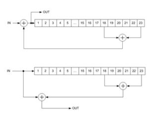
One problem with self-synchronizing scramblers is that an error in the received data pattern can result in multiple errors in the de-scrambled data. This is called error propagation.
