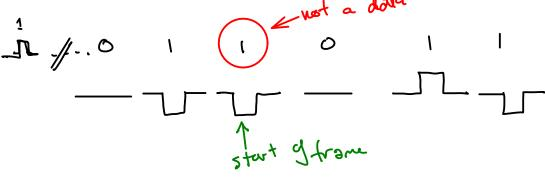
**Exercise 2**: Preambles such as this allow multiple transmission formats to be used in a backwards-compatible way. What might be some disadvantages of using such a preamble? *Hint:* to be decoded by old ("legacy") devices the preamble must be transmitted at the lowest possible data rate. This can be 100 times slower than the fastest devices.
