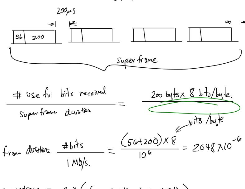
superfrance =  $4 \times (\text{france auxation} + \text{gap auxation})$ =  $4 \times (2048 \times 10^{-6} + 200 \times 10^{-6}) = 8992 \mu s$ troughput =  $\frac{200 \times 8}{8992 \times 10^{-6}} = 178 \text{ kb/s}$ if 10% are "lost" twoysput =  $178 \cdot (1-10\%) \approx 160 \text{ kb/s}$ .
