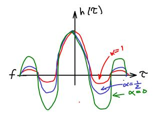
Larger values of excess bandwidth (wider bandwidth channels) results in less "ringing" of the impulse response which in turn reduces the amount of ISI near the sampling point of the next symbol. This makes the receiver less sensitive to errors in its timing of the sampling point.
