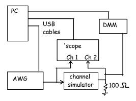
As shown in the photo below, the AWG and the Channel 1 probes should be connected to the channel simulator<sup>5</sup> terminals marked IN and GND and the 100  $\Omega$  resistor, the Channel 2 probe and the DMM probes to the terminals marked OUT and GND. All the switches on the channel simulator should in the down position<sup>6</sup>.
